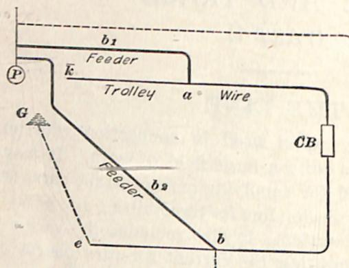
in the track return than in the overhead feeder. A ground wire run from some point on the rail in the neighborhood of  $b$ , or even from the end  $e$  to the ground bus-bar at the power station, would greatly improve the service.
